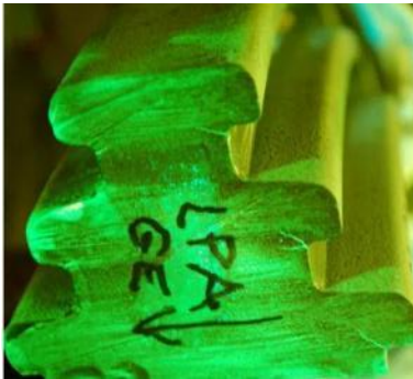
Fig. SCC of a Steam Turbine Disk Dovetail
