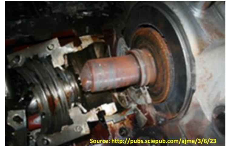
Fig. Damage of Turbine Shaft
