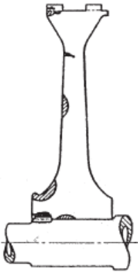
Fig. Typical Locations of SCC Damages (LP turbine discs)
