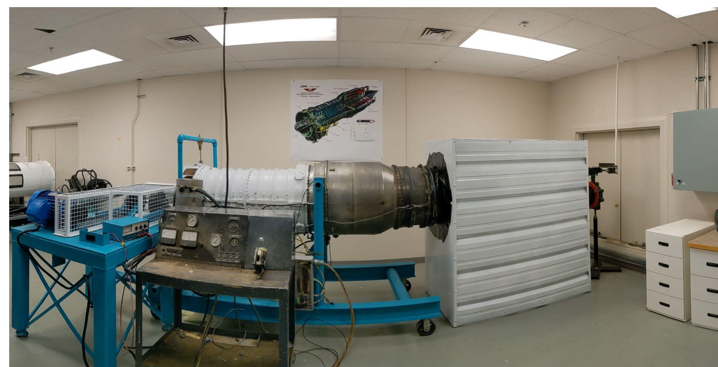
Figure 3. J34 Test platform and Test Stand
